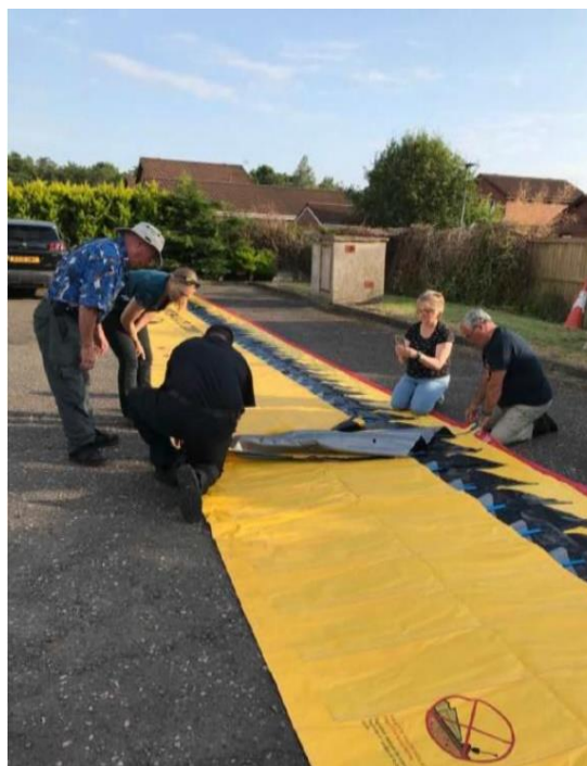
Figure 16 Testing of Watergate System by Local Flood Group (TIDECO) in Tillicoultry – 29th June 2021
