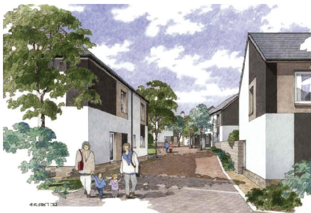
Buildings framing a junction on shared surface, naturally slowing vehicles, and making a pedestrian friendly environment. Windows face the road from both sides to provide passive surveillance - Polnoon Masterplan, McTaggart Mickel
