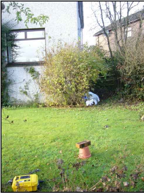
Figure 5.30: Photograph of Vibration Monitoring Equipment at 20 Ladywood, Clackmannan
