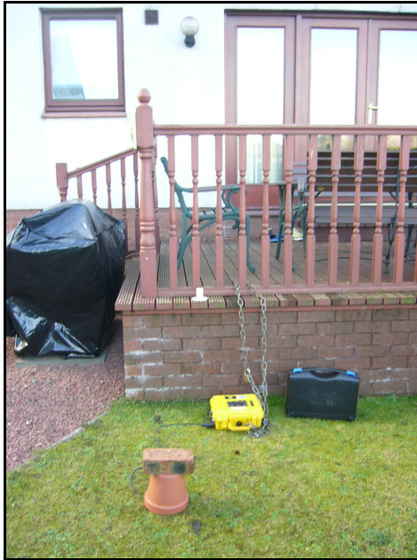
Figure 5.15: Photograph of Vibration Monitoring Equipment at 25 Brucefield Crescent, Clackmannan
